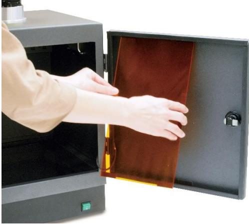
Remove the filter shield from the door and turn it around. The magnets should be facing you.
