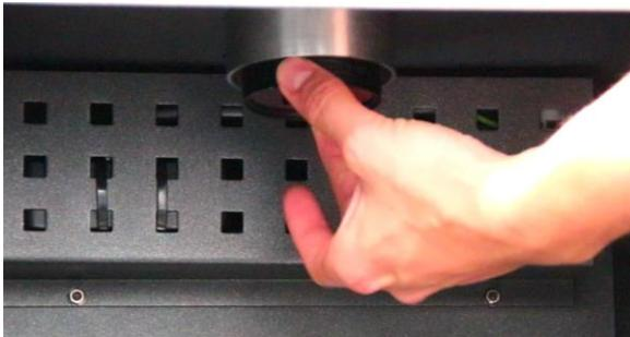
After zooming out, you can remove the amber filter from the lens, by using 2 fingers, as shown in the left image. The amber filter should now be stored in a safe, clean storage space and be added as soon as the image is taken. To add the filter to the lens, just hold the amber filter close to the lens and the magnet will pull the amber filter to the correct position.
