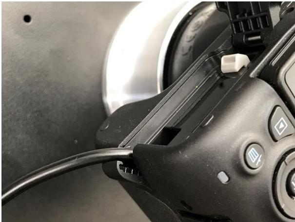
3. Close the battery compartment completely. Please put the cable in the cable channel. Please note: the camera will not turn on if the battery compartment is not completely closed.
