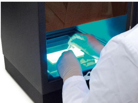
Turn on the transilluminator. Now look through the filter shield and excise the DNA band using a scalpel or our FastGene® Agarose Gel Band Cutter (FG-830)
