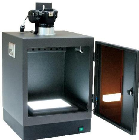
Add the white LED transilluminator to the central area of the Blue/Green LED Transilluminator as shown in the picture. Turn the switch to battery. Make sure that the transilluminator is charged, otherwise connect the transilluminator to a power source using the USB charger cable. Select the required brightness by pressing the switch button. Record your image.
