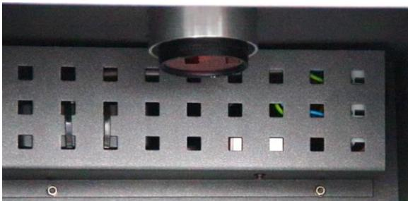
Extend the lens barrel by zooming out. The lens is now exposed and the filter is ready to be removed. The filter is held in place using a magnetic filter holder. After removing the filter, add the white light source (e.g. our white light transilluminator FG-07)
