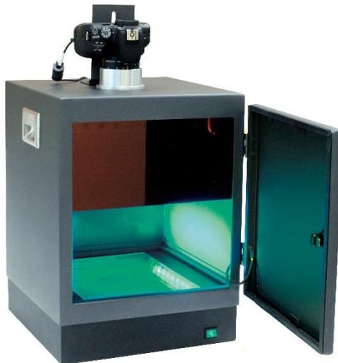
Attach the filter shield to the magnets inside the box.
